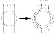
i.e., superconductors are *perfect* diamagnets
