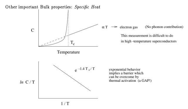
The entropy of the S.C. state is smaller than in the normal state.
