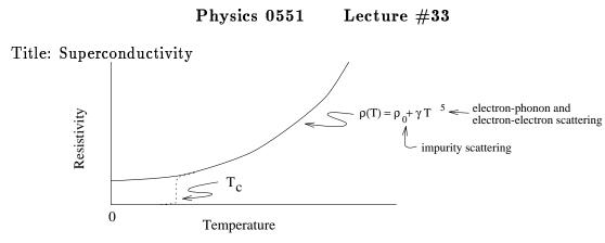
Superconductors are unusual for a variety of reasons. The first observations were made in 1911 by Kamerlingh Onnes (Denmark) on the low temperature behavior of Hg (mercury) and he observed a complete absence of  $\rho$  in the vicinity of 4°K.
